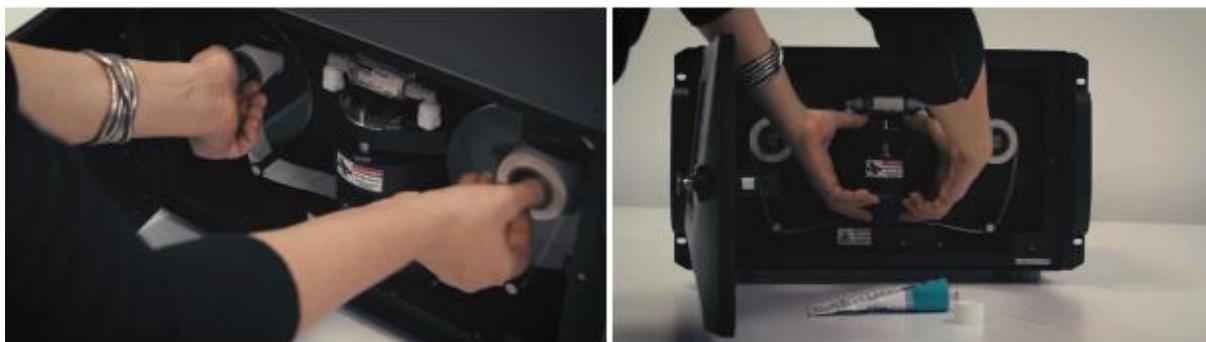
6. Using thumb and fingers on both sides of the optical chamber, lift the chamber upwards against its springs.
