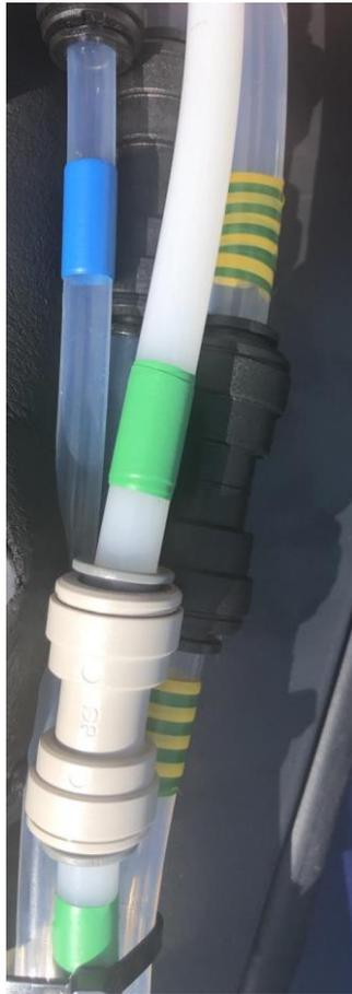
Figure 8.3 – PM Sample lines for connection of flow meter and HEPA filter.
