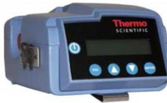
Figure 8.1 – Thermo PDr 1500, PM<sub>2.5</sub> Monitor
