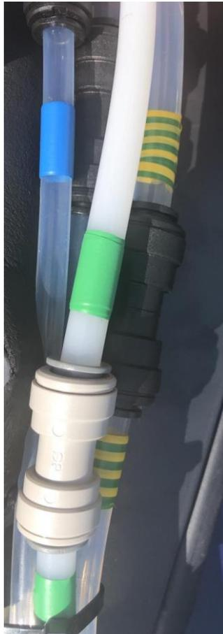
Figure 7.3 – PM sample lines for connection of flow meter and HEPA filter
