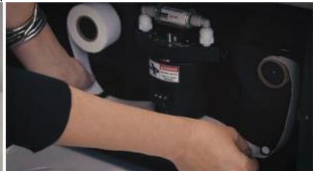
13. Make sure that the tape is fed beneath both the left and the right guide posts and passes under the optical chamber.
