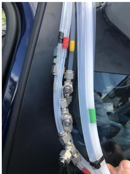
Figure 1.3 – Calibration port for 211G (RED)
