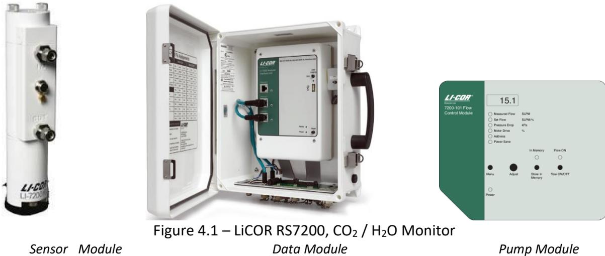
The LiCor monitor measures CO<sub>2</sub> and H<sub>2</sub>O by infrared absorption and can be found towards the rear of the cars, in three modules. The pump module which samples the air at up to 10 lpm, the data module which manages the signals and communications and the sensor module which actually makes the measurements. There is no screen on this instrument, so proper operation should be confirmed online.
