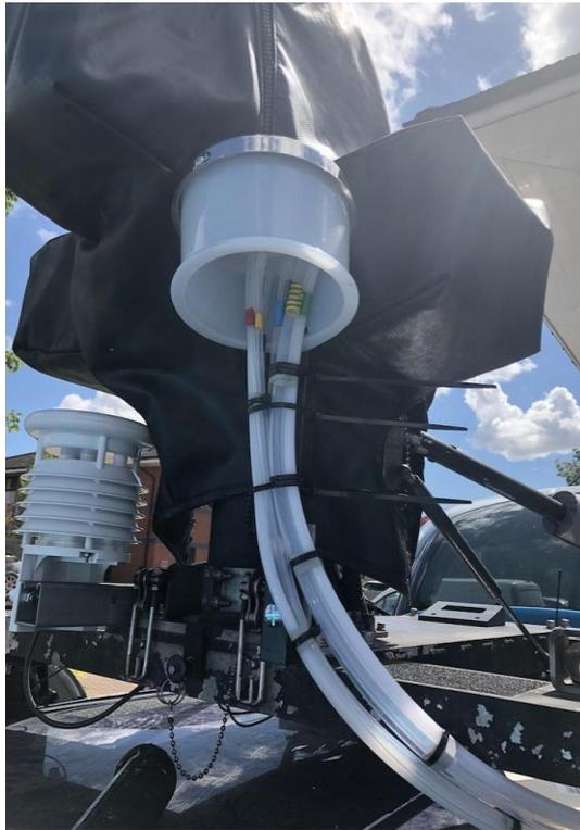
Figure 8 – Sample Inlet Head for Gas and Particles and Met Sensor on roof bar
