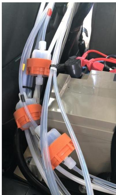
Figure 1.5 Gas Monitor Particulate Filters
