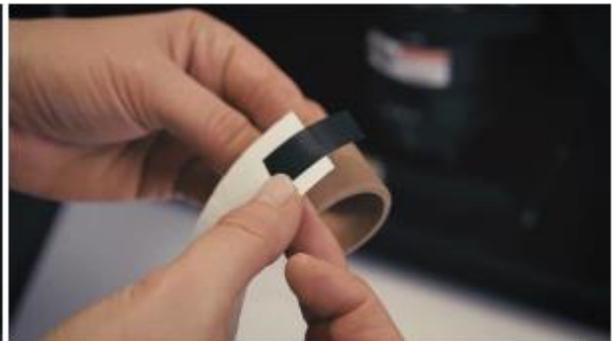
10. Make sure the roll is correctly oriented – the tape must unroll from the left-hand side.
