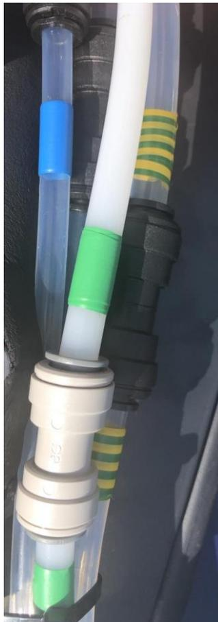
Figure 5.3 - PM Sample Lines for attachment of flow meter and HEPA filter (vertical on car)
